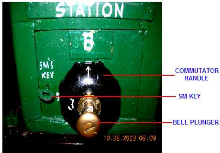
Fig: 4.4 COMMUTATOR HANDLE AND BELL PLUNGER
