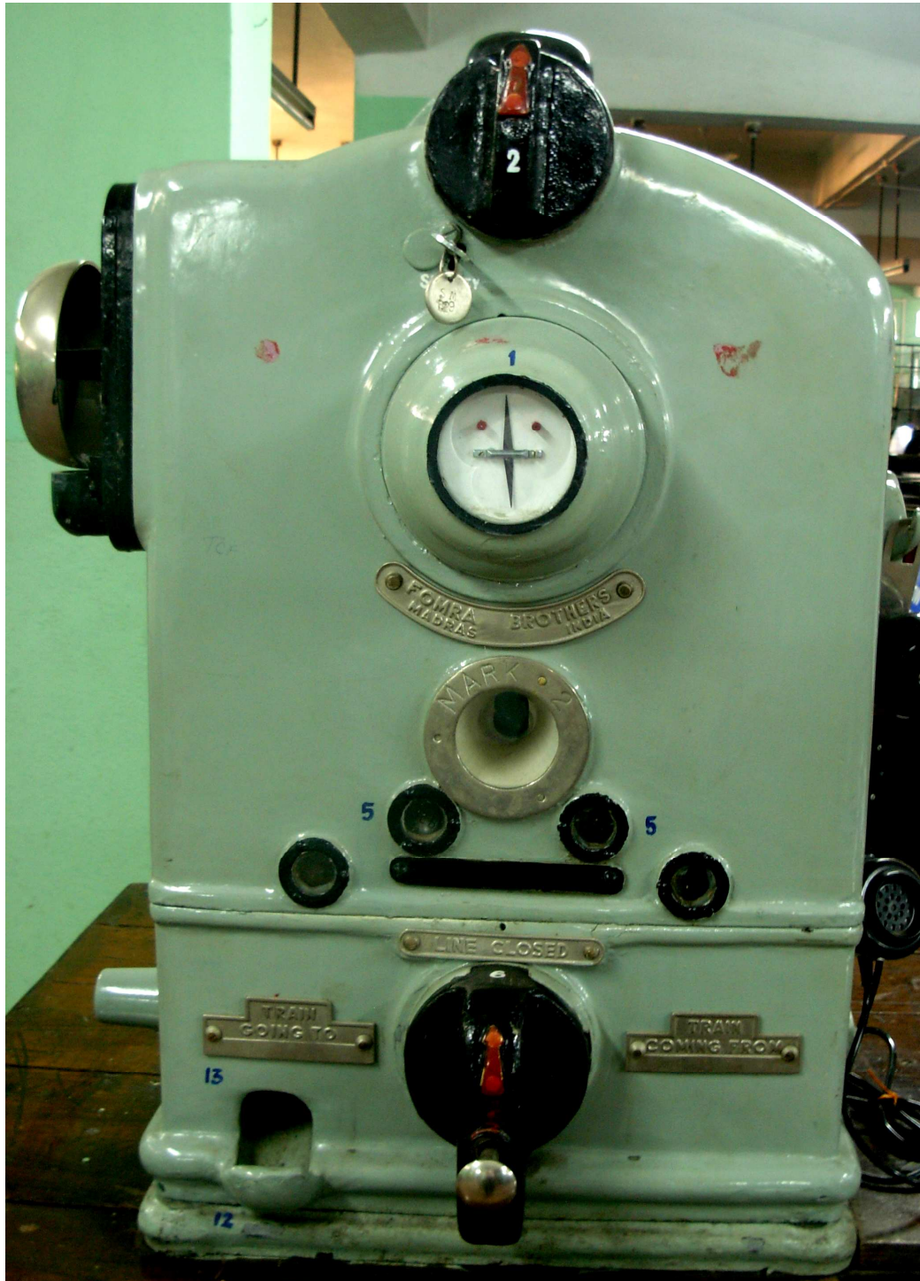
Fig. 2.2 NT BALL TOKEN BLOCK INSTRUMENT (FRONT VIEW)
